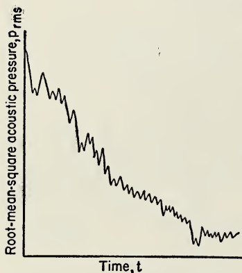
FIG. 12-3. Typical variation of acoustic pressure with the time during the decay period. Many modes of room vibration are present.
